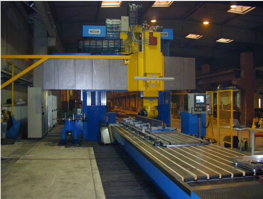
Modular designed portal milling machine for machining of large surfaces – e.g. blocks or sheets
