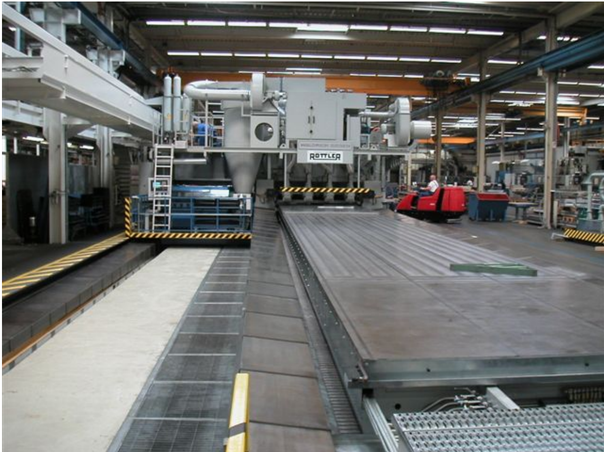
The PFGA X-32 milling machine for high-speed aluminum processing is modularly designed and hence easily to be maintained.
